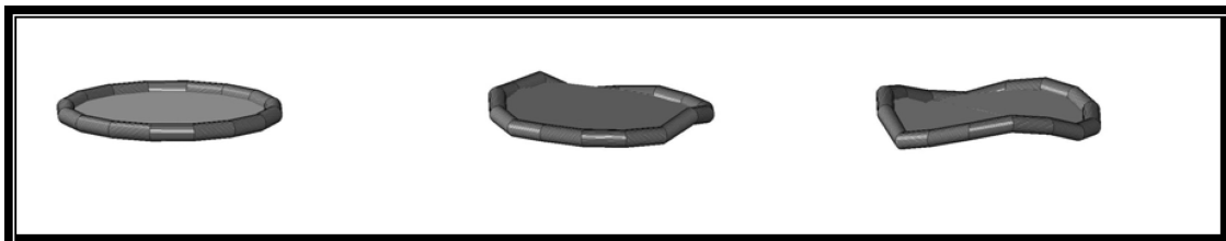
Fig. 3 Experimentally identified mode shapes of an inflated torus with attached membrane mirror (top). The torus is shown at rest (left) and vibrating at the first and second out-of-plane modes (middle and right).
